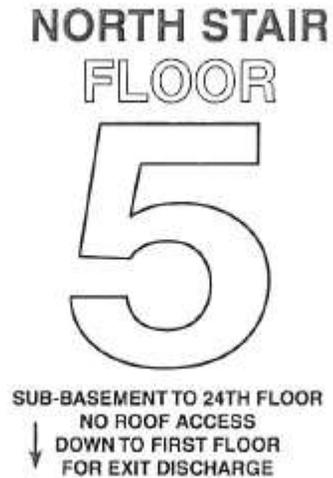
FIGURE A.7.2.2.5.4 Example of a Stairway Marking Sign.
