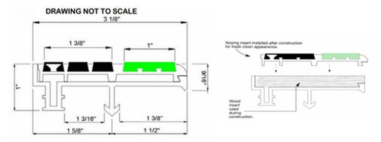
These high quality photoluminescent and slip resistant stair nosings provide an exit path marking and safety egress system that meets all building & fire codes in the US & Canada. These stair nosings also meet the requirements of NFPA 101, The Life Safety Code. The use of heat treated and corrosion resistant aluminum assures superior resistance to wear under heavy pedestrian use. EverGlow surfaces are easy to clean and maintain.
