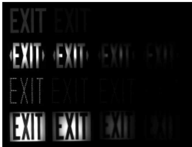
Computer simulation of the visibility of exit signs in smoke. From top to bottom, the types of exit signs shown are electroluminescent stencil, compact fluorescent stencil, LED matrix, and incandescent panel. From left to right, the simulation shows the original sign (no smoke) and the sign "viewed" from 6.56 feet (2 meters), 16.4 feet (5 meters), and 23.0 feet (7 meters) in gray smoke. The brightnesses of the different types of signs were balanced to make them roughly the same in the clear-air condition; thus the apparent brightnesses of the different sign types should not be compared with each other.
