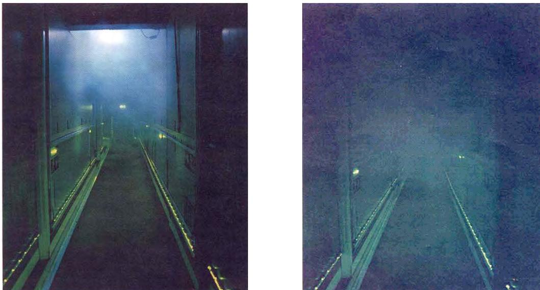
**Figure 10: LED system progressively obscured by simulated smoke, BRE study [24]**
