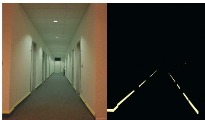
Interior Corridor marked along the baseboard.
